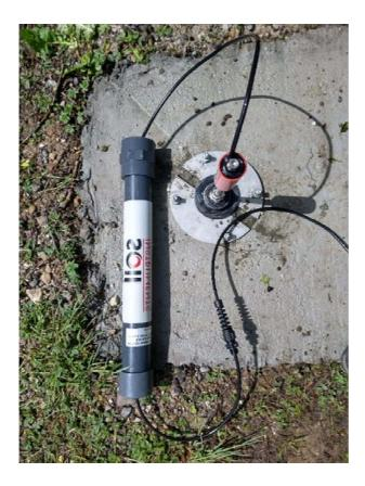
Fit the cover to the head, refit the gland to the cover and tighten the cable gland nut to seal the cable.
