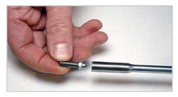
Tighten the reading datum fully into the rod connector and withdraw the nut spinner.
