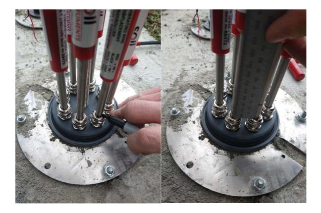
Carefully extend the transducer to its desired starting position and tighten the securing gland using the gland tightening tool whilst holding the transducer in position, hold tightly to prevent the transducer from rotating whilst tightening.
