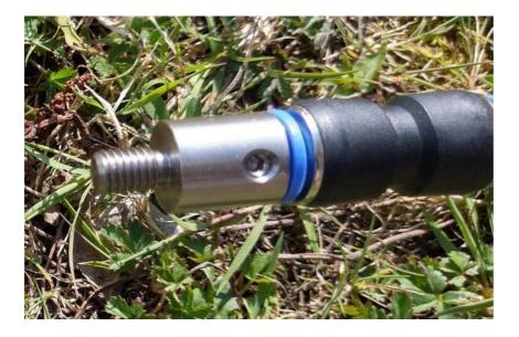
Pull the release ring back on the inline connector where the red nylon tube enters the inline connector.
