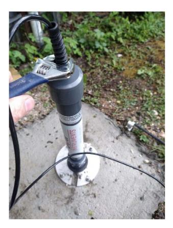
Remove the sealing caps from the rod positions to be read.
