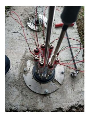
Do not over tighten, max 3 Nm
