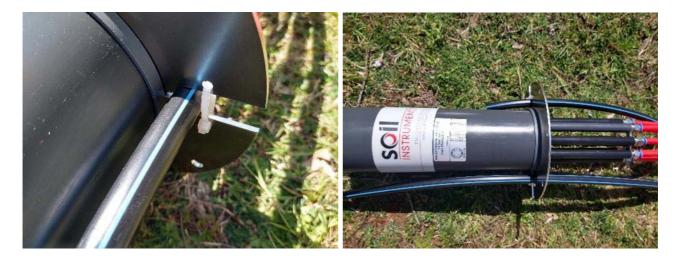
If the head is to be secured to a hard surface of rock or concrete the surface should be flat and perpendicular to the borehole.
