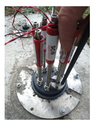
Set the remaining transducers and record the initial reading from each transducer, noting the serial number of the transducer and the rod position.
