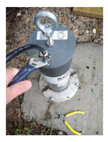
Thread the seal nut down the threaded bar with its seal towards the cap.
