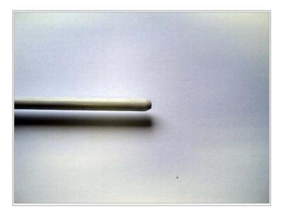
The GRP should protrude from the red nylon tube by 35mm.
